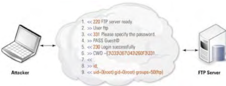
Figure 1 FTP buffer overflow attack
