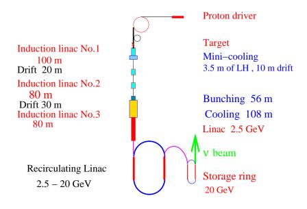
Figure 2.2: Schematic of the neutrino factory-Study II version.
