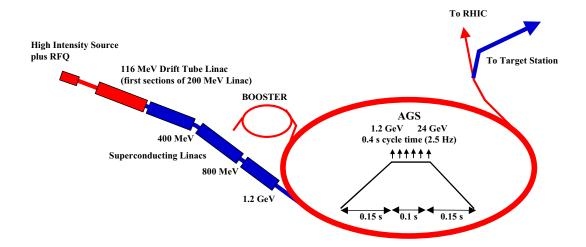
Figure 4.1: AGS proton driver layout.
