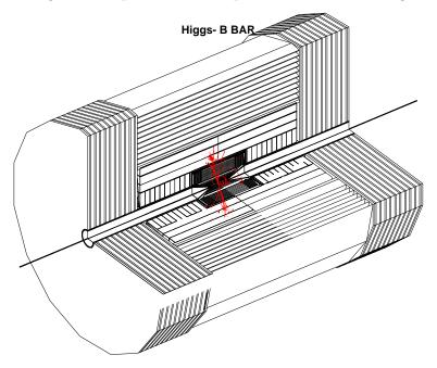
Figure 5.7: Cut view of a strawman detector in GEANT for the Higgs factory with a Higgs  $\rightarrow b\bar{b}$  event superimposed. No backgrounds shown. The tungsten cones on either side of the interaction region mask out a 20deg area.
