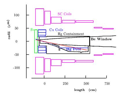
Figure 4.3: Target, capture solenoids and mercury containment.
