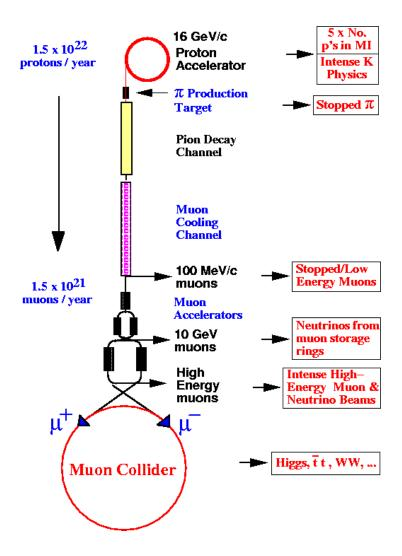
Figure 5.2: Schematic of a muon collider.
