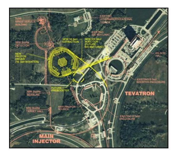
Figure 4.2: FNAL proton driver layout.
