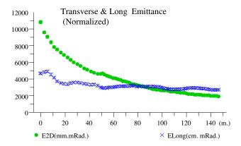
Figure 4.6: The longitudinal and transverse emittances, obtained with the Geant4 simulation code, as a function of channel length. The last lattice (2,3) was extended by  $\approx 20$  m to investigate the ultimate performance of the cooling channel.
