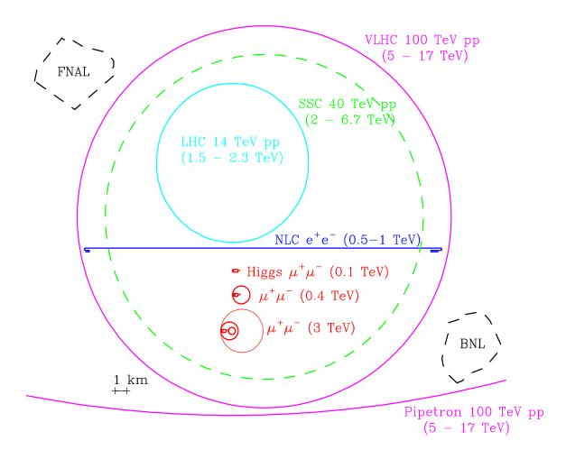
Figure 5.1: Comparative sizes of various proposed high energy colliders compared with the FNAL and BNL sites. The energies in parentheses give for lepton colliders their CoM energies and for hadron colliders the approximate range of CoM energies attainable for hard parton-parton collisions.
