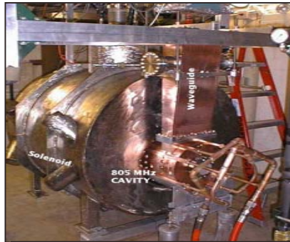
5T Cooling Channel Solenoid – LBNL & Open Cell NCRF Cavity operated at Lab G – FNAL
