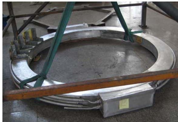
Fig. 9. Cold-mass assembly for large test coil at ICST.
