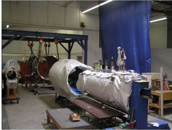
Fig. 7. Second spectrometer solenoid being assembled at Wang NMR.
