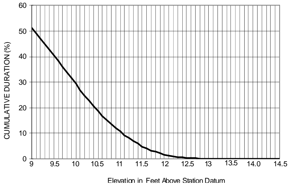
Figure 12B. Duration of Inundation for High Water at the Presidio Between 1922 and 1984
