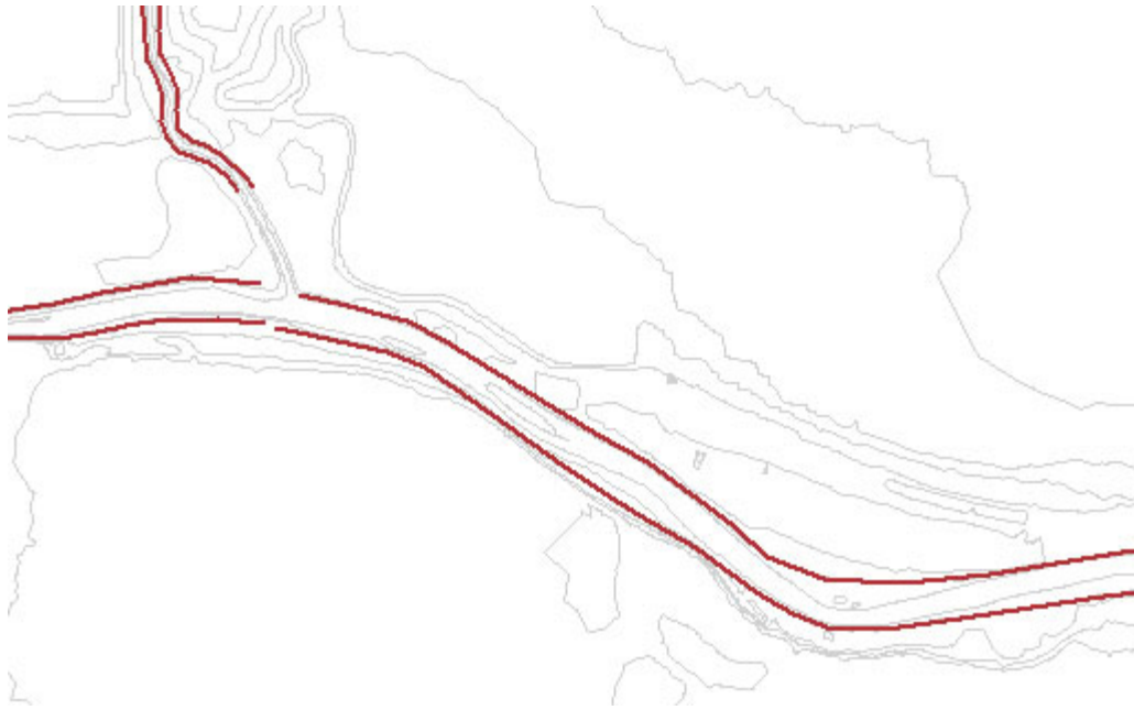
Figure 7-9. Bank lines delineate the main channel from the overbank areas.
