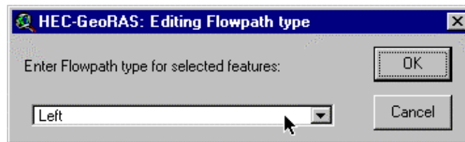
Figure 6-8. Each flow path must have an identifier of "Left", "Channel", or "Right".
