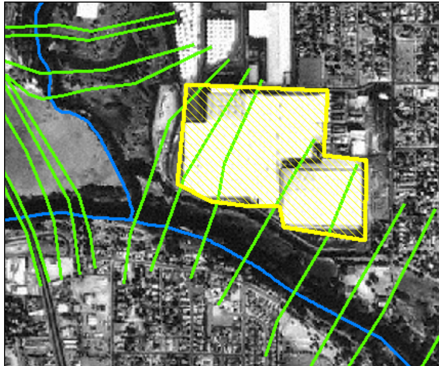
Figure 8-24. An obstruction (building) to flow in the floodplain is represented using a blocked obstruction.
