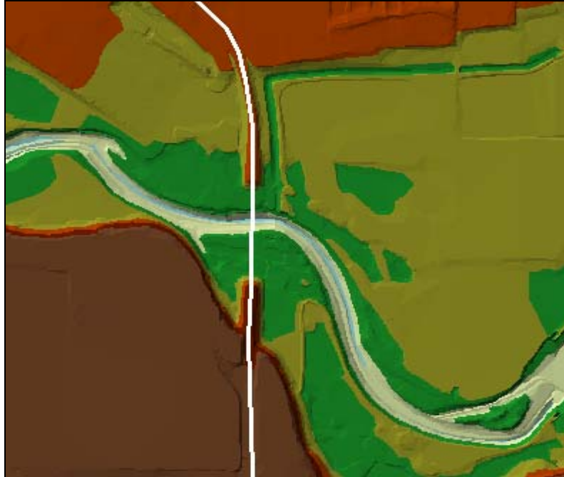
Figure 8-20. Locate bridge cut lines at the road centerline to capture high ground.
