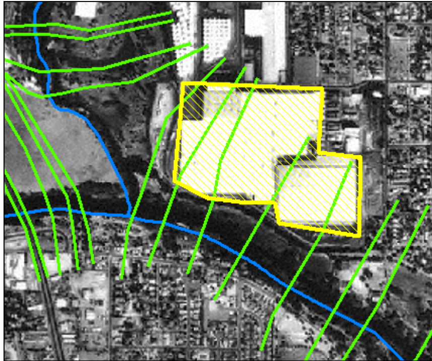
Figure 8-24. An obstruction (building) to flow in the floodplain is represented here using a blocked obstruction.
