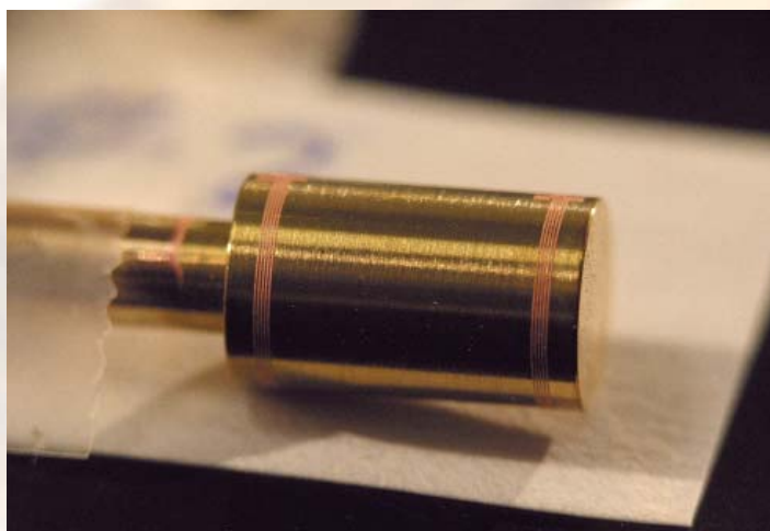
Figure 3. 6\text{-mm} -OD brass mandrel patterned with copper to simulate "Hohlraum" heater wires.
