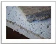
Perlite used in ceiling tiles dampens noise.
