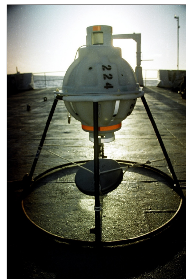
An array of three inverted echo sounders (IES) equipped with pressure gauges and one IES with a current meter were moored on the sea floor this past March 2009 along 34.5°S. Data from the array were gathered for the first time in August 2009 from the Argentine research vessel Puerto Deseado .
