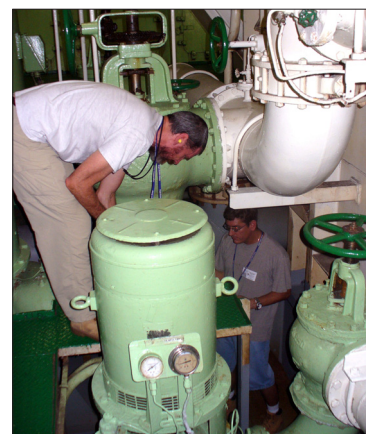
Following the installation of a thermosalinograph aboard the Barcelona Express , Kevin Sullivan and Denis Pierrot perform a logistical survey to prepare the vessel for the installation of a pCO 2 system that will gather ocean carbon data.
