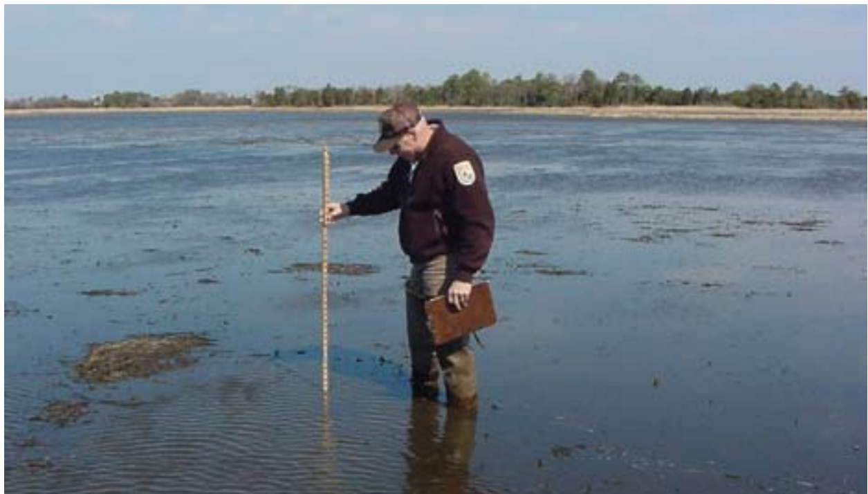
Measuring water depths for bathymetric map of impoundment at Prime Hook NWR
