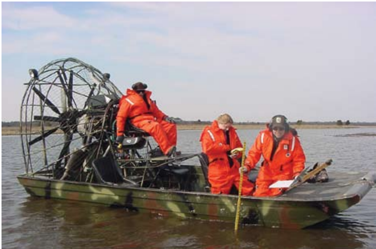
Collecting impoundment bathymetric data at Prime Hook NWR
