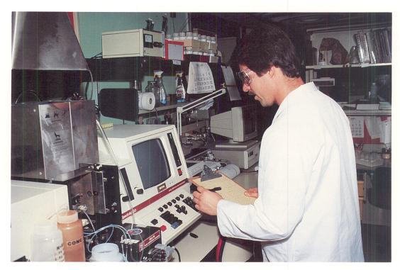
Plasma emission spectrophotometry is often used when a toxic substance is suspected, but the nature of the agent is unknown.
