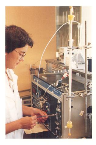
High-performance liquid chromatographs can be used for direct analysis, molecular separations, or the cleanup of extracts from samples collected in the field. There may be an additional charge for preparing sample extracts for analysis.
