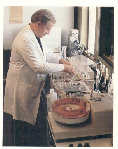
The use of autoanalyzers provides rapid and highly sensitive water chemistry determinations.
