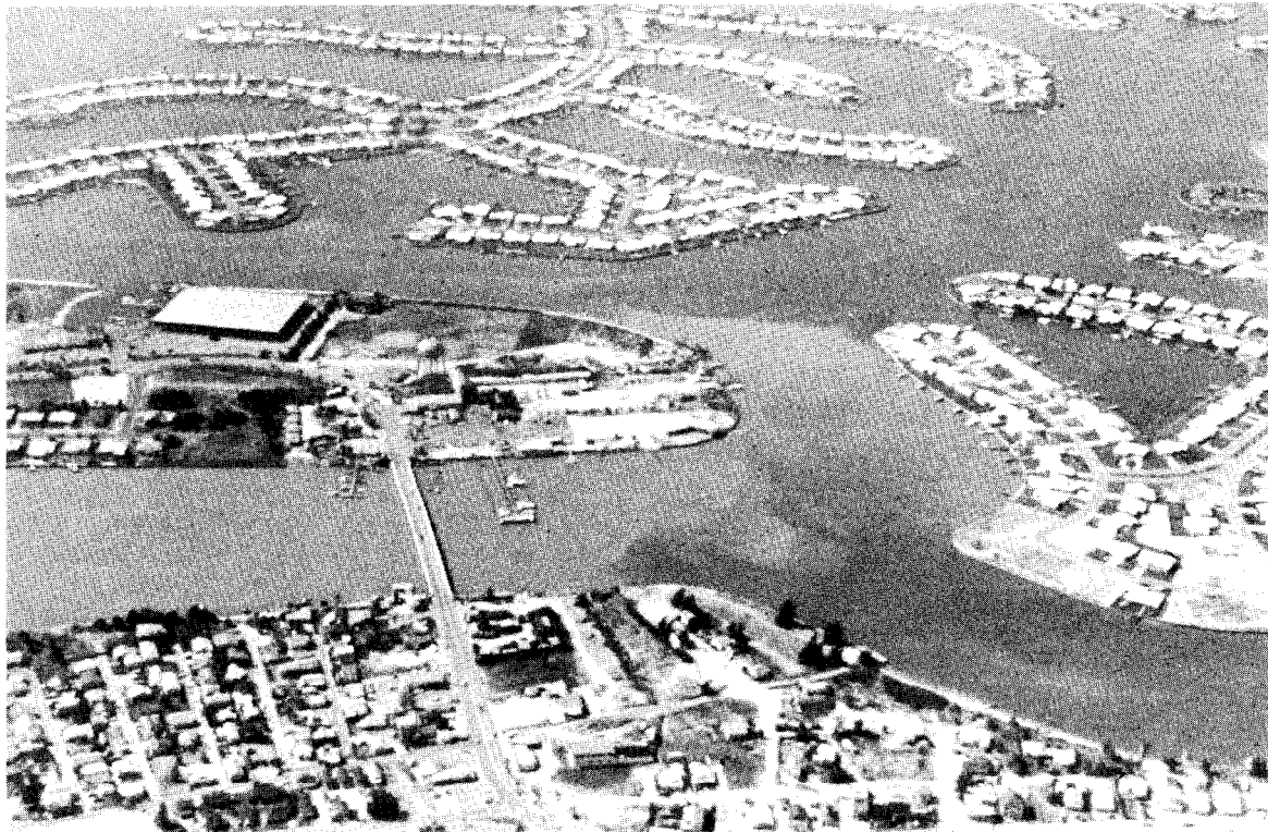
Figure 27. Dredged and filled areas in Boca Ciega Bay (photo by M. J. Durako).
