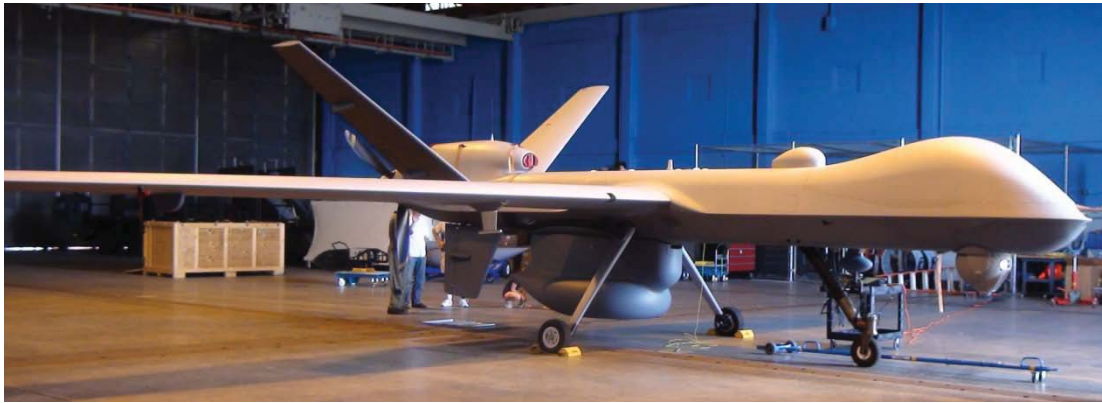
Figure 1. Guardian, the maritime variant of the Predator B. Source: CBP Sierra Vista, Arizona, NASOC
