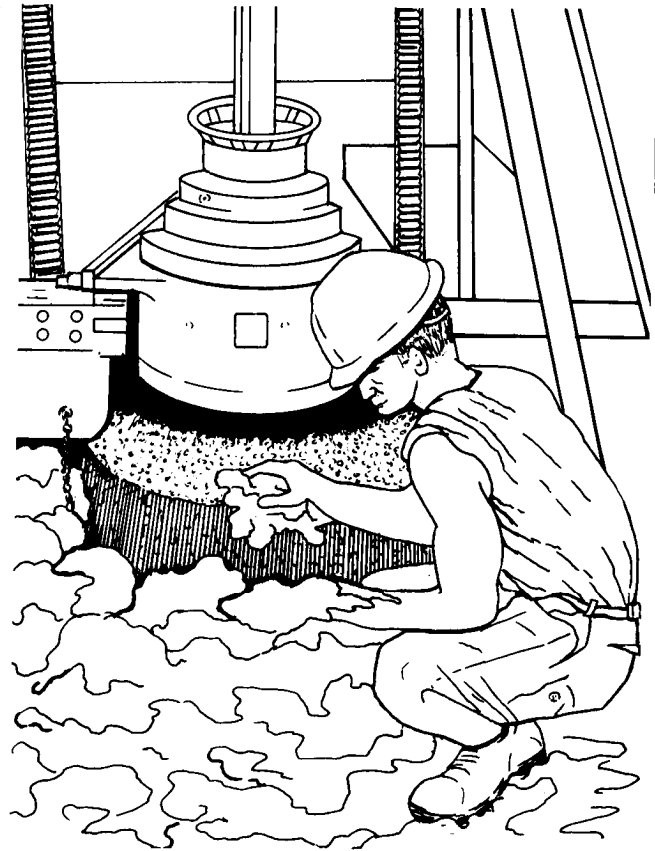
Figure 5-15. Foam from the well
