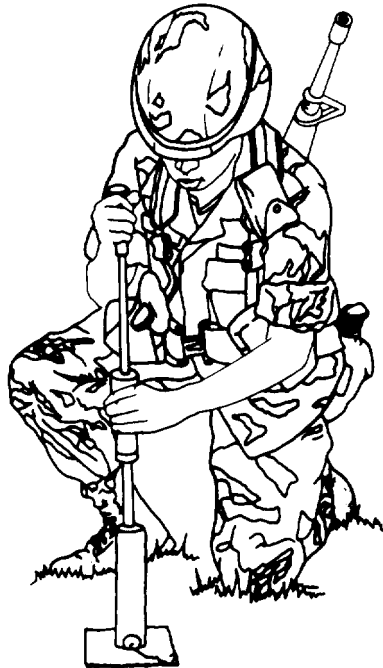
Figure E-11. Applying hammer blows with remolding equipment
