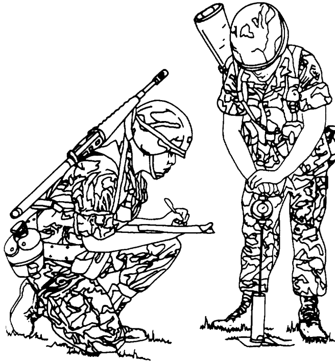
Figure E-10. Measuring cone index in a remolding cylinder
