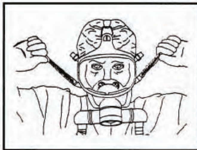
Figure 3-10. Tightening lower straps
