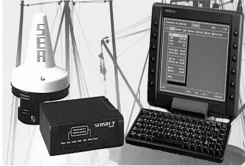
Figure 5-2. INMARSAT C Above/Below Deck Equipment
