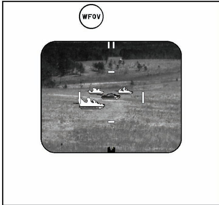
Figure E-30. Counteracting man-made clutter Step 2—adjust contrast.
