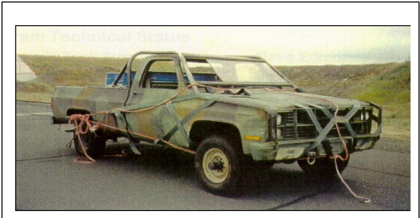
Figure L-14. Vehicle Entrapped in a PVAB
