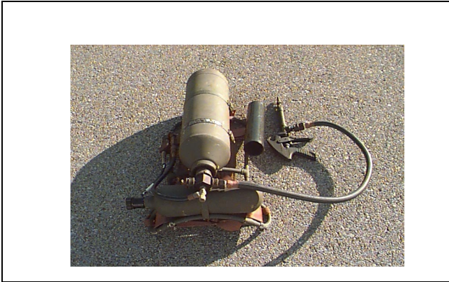
Figure L-10. M33A1 Riot Control Dispenser Filled With CS or CR
