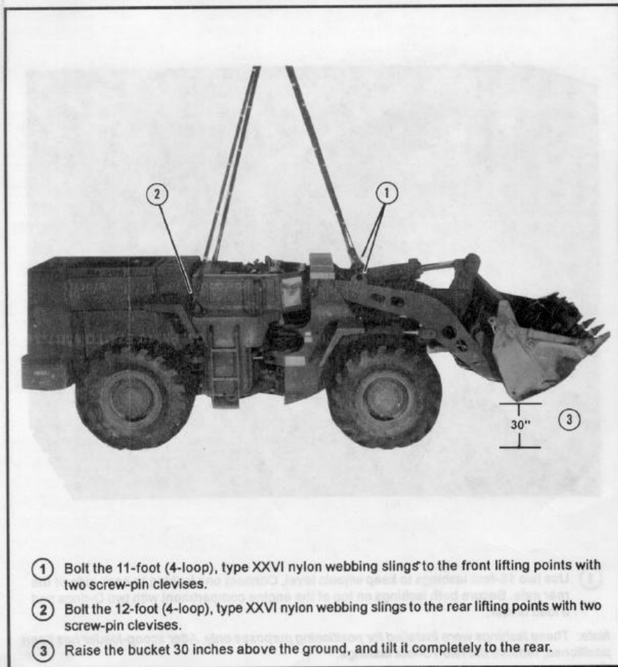
Figure 5-6. Lifting slings installed
