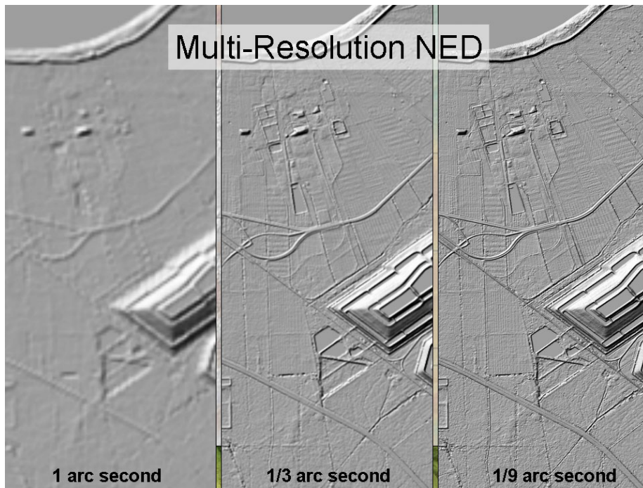
Figure 16. Multi-resolution elevation data in the National Elevation Dataset
