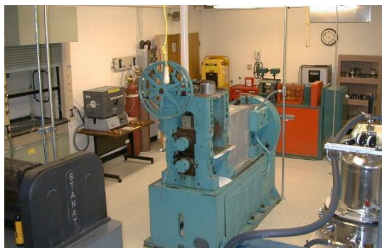
Figure 7. Rolling mill for hot or cold rolling.
