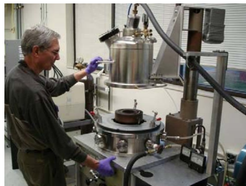
Figure 5. Arc melter for consolidation and metal casting.
