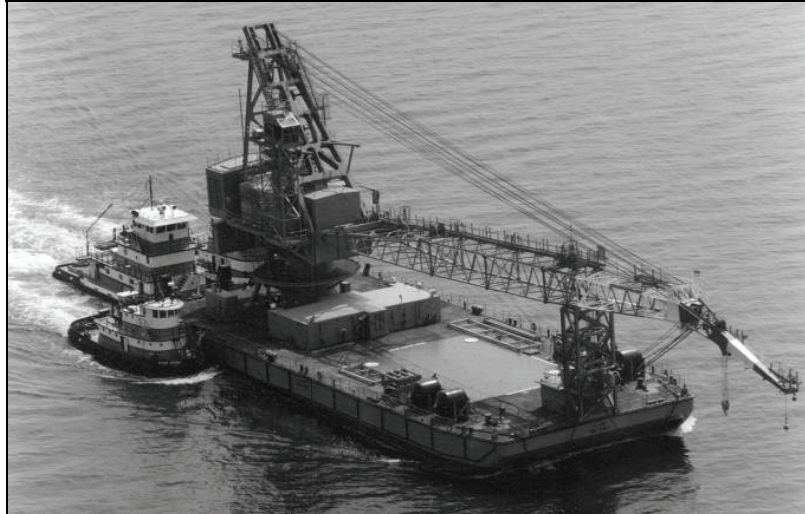
Figure 2-9. Barge Derrick, 115 Ton
