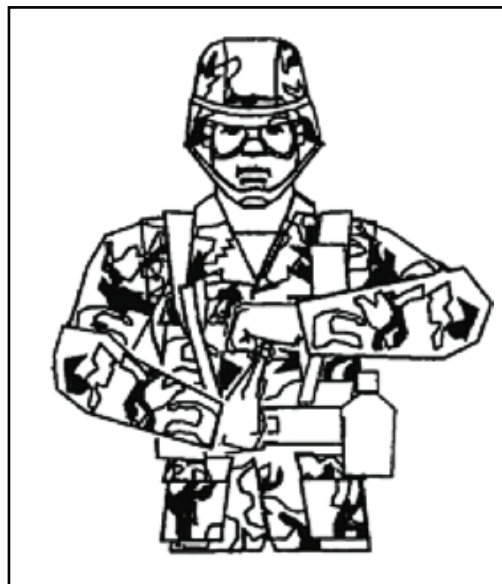
Figure A-27. Load has not been released
