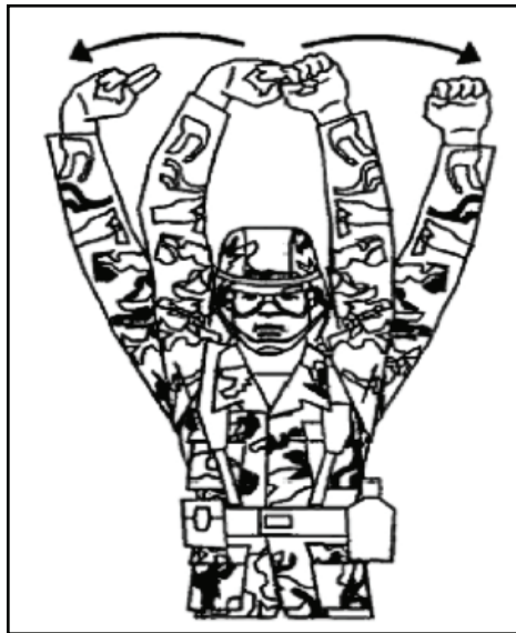
Figure A-24. Disconnect auxiliary power unit (day)
