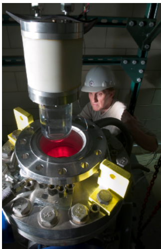
Figure I-2: The insertion of the inner vessel/bellows assembly into the pressure vessel in the MINOS area at Fermilab (left), and the complete apparatus partially enclosed during the stacking of the polyethylene neutron shielding.
