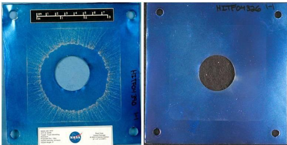
Figure 4.— Comparison of ejecta plate damages following impact of 0.3175 cm diameter aluminum spheres on a monolithic aluminum outer bumper (left) and stainless steel foam outer bumper (right) at hypervelocity (approximately 6.8 km/s).
