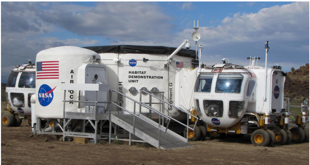
Figure 1.— The HDU1-PEM (center) with two docked space exploration rovers. The main HDU-PEM volume includes several workstations. Three circular ports below “Habitat Demonstration Unit” are the antechamber doors that provide access directly into the GeoLab glovebox.
