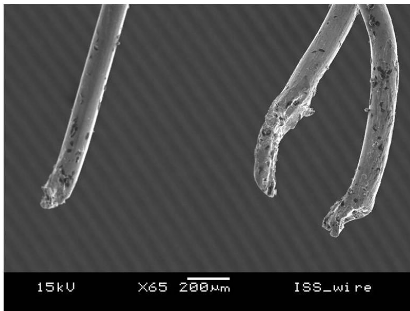
Figure 3.— Three wires exhibiting melt.
