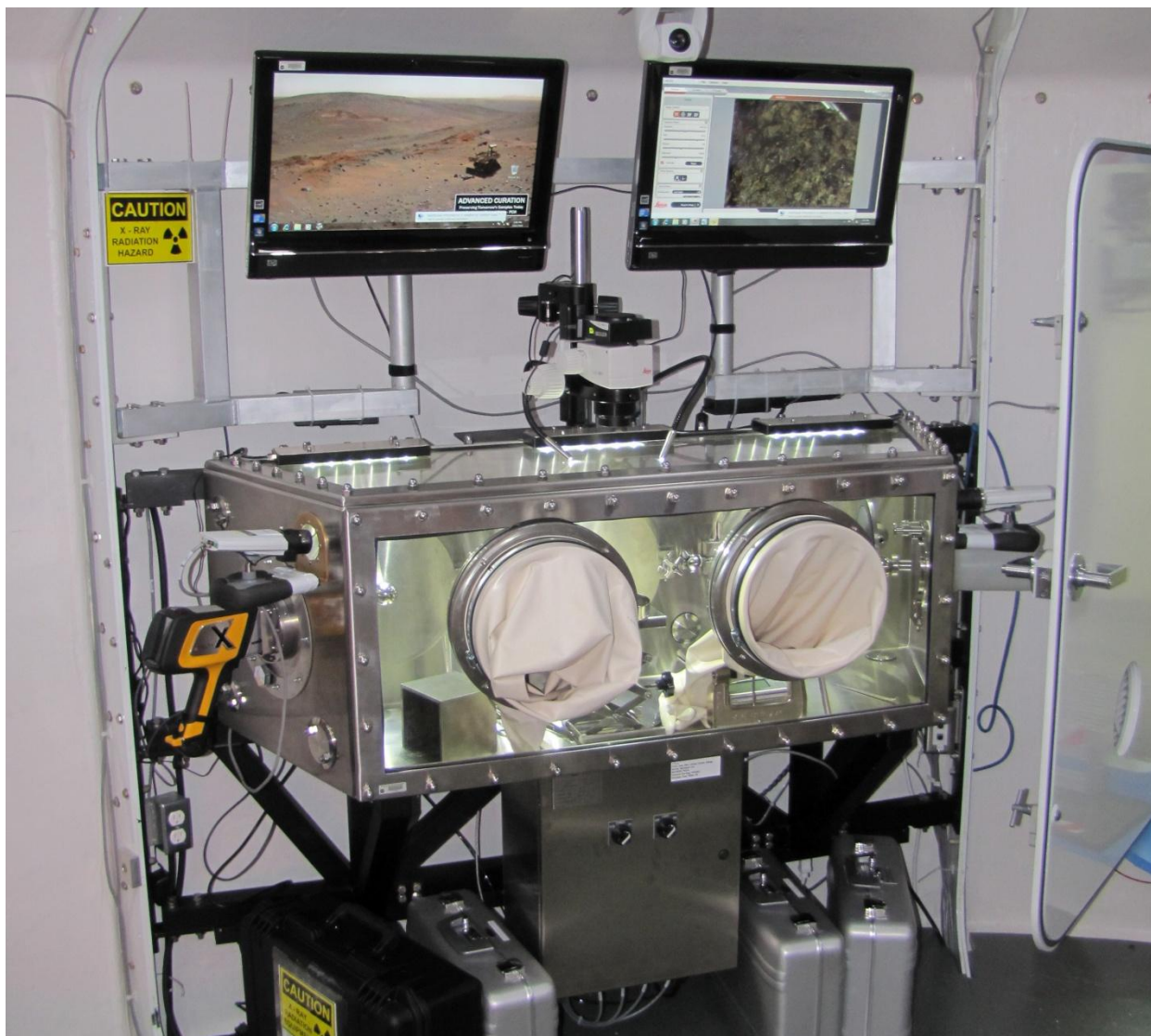
Figure 2.— GeoLab integrated into the HDU1-PEM. The suite of instruments included a handheld XRF analyzer (far left), stereo microscope (center, above glovebox), network cameras, and touchscreen computers.
