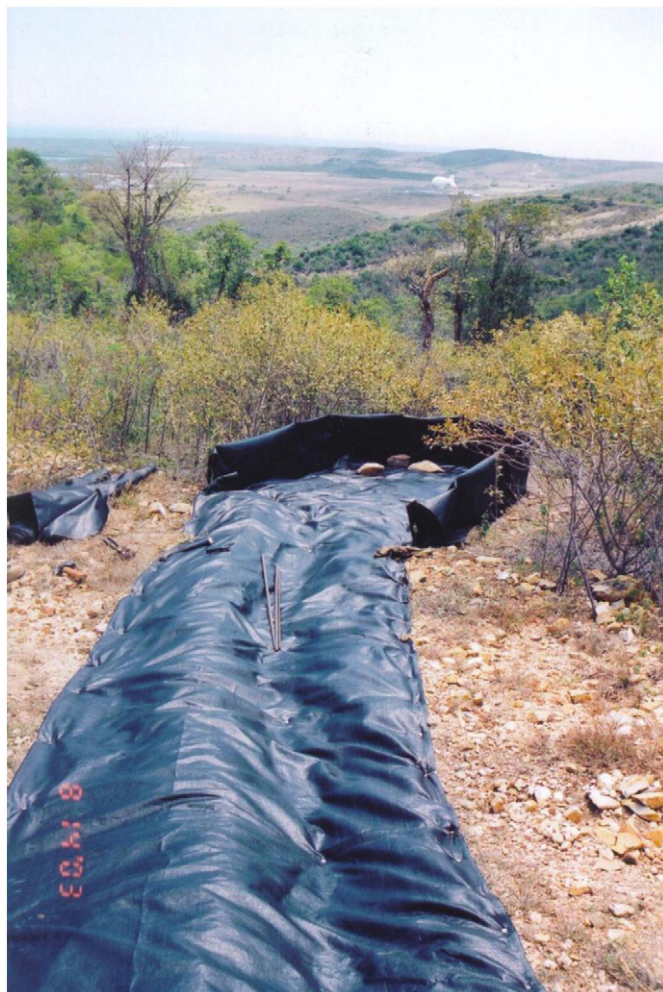
Fig. 2. An example of a sediment trap used to measure sediment production rates (Road-O-Top). Fabric floor was used to protect pre-existing road cross-drains and to facilitate the extraction of eroded material.
