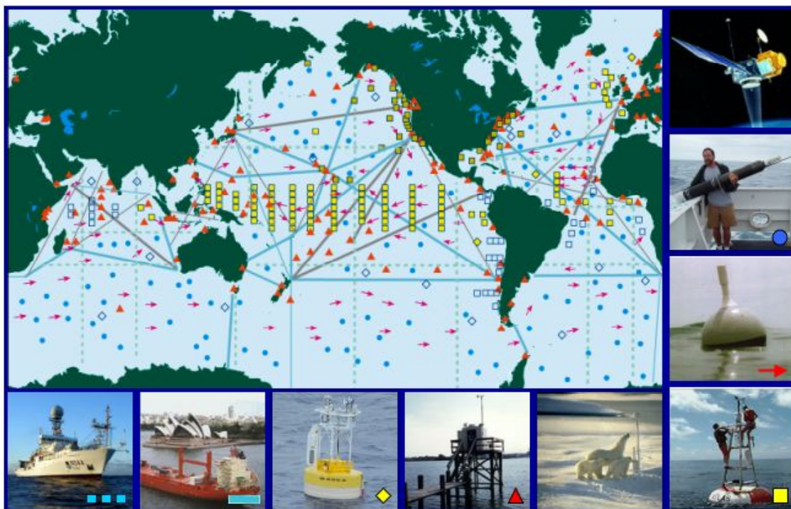
Figure 1. The subsystems that make up the Sustained Ocean Observing System for Climate are illustrated from lower left to upper right: Dedicated Ships, Ships of Opportunity, Ocean Reference Stations, Tide Gauge Stations, Arctic Ocean Observing Network, Tropical Moored Buoy Network, Surface Drifting Buoys, Argo Profiling Floats, and Continuous Satellite Missions for sea surface temperature, sea surface height, surface vector winds, ocean color, and sea ice. Not illustrated are the Data & Assimilation Subsystems, and Management & Product Delivery, which provide the overarching system integration.
