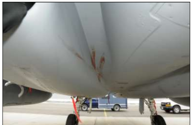
Under-belly of aircraft after a bird strike February 2011 (Photo by Senior Master Sgt. Robert Sabonis)
