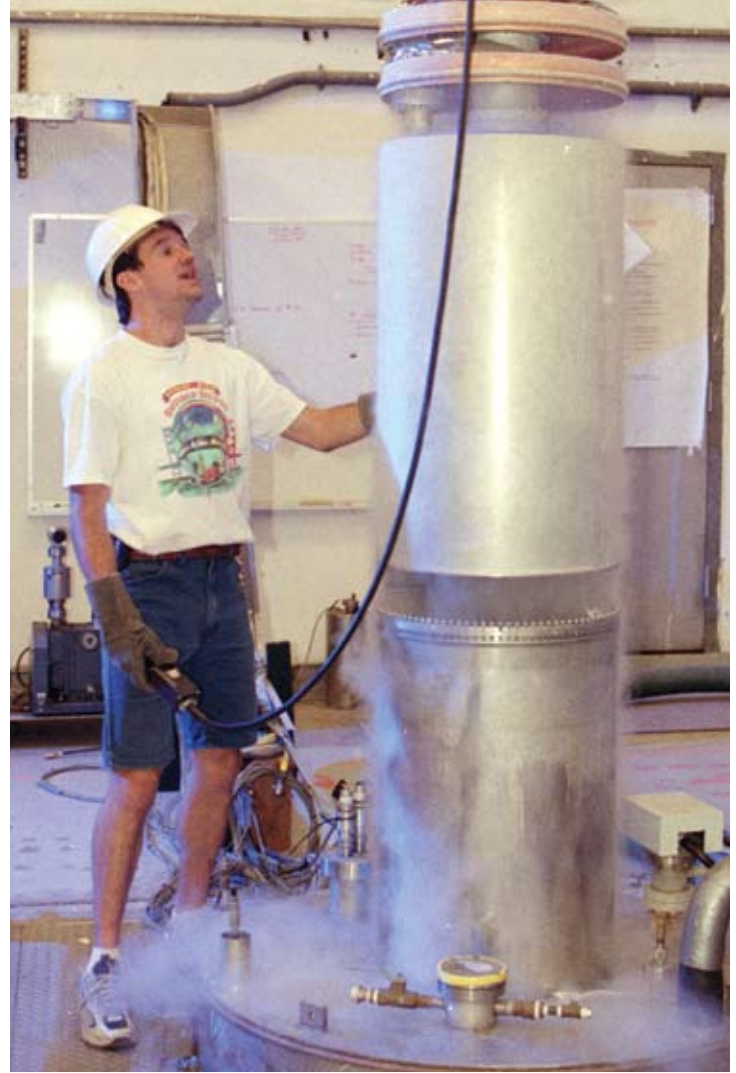
Livermore physicist Darin Kinion guides the experimental apparatus containing the microwave cavity and superconducting quantum interference device (SQUID) amplifiers into the cavity of a superconducting electromagnet for the Axion Dark Matter Experiment (ADMX). The disks on top of the ADMX device are thermal shields.
