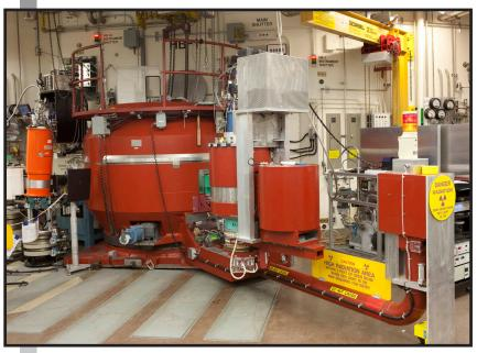
investigating small samples and weak scattering in specific areas of energymomentum space. The sample goniometers and a full software implementation of the three-dimensional sample orientation matrix allow measurements outside the traditional singlescattering plane. The unique capability of HB-1 is the polarized configuration for studies of excitations, phase transitions,
