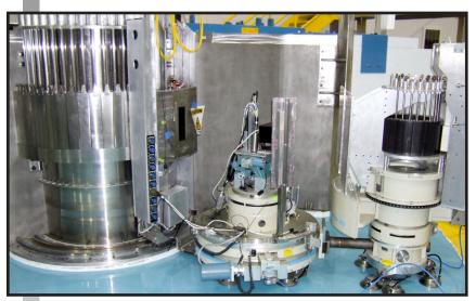
by CG-4C's vertically focusing monochromator PG (002). To enhance accommodation of strong magnetic fields at the sample position and to simplify future polarization analysis, the amount of ferromagnetic material has been minimized in the construction of this instrument.
