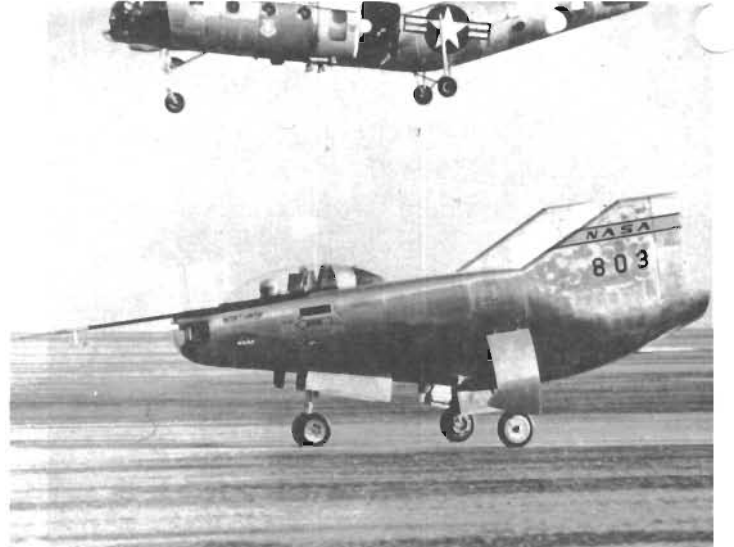
The M2F2, the first of the "lifting body" vehicles, marked the beginning of a six-year program gathering data for designs of hypersonic aircraft and earth re-entering spacecraft such as the Space Shuttle.
