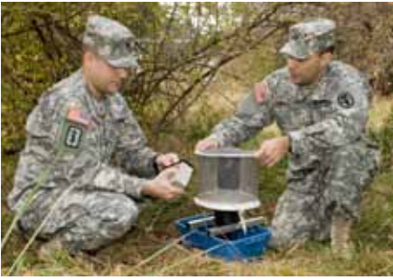
Entomologists, CPT Michael Desena (left) and CPT Jorge Lopez (right), routinely monitor mosquito populations. The mosquito light trap captures mosquitoes which are identified and tested for the presence of disease pathogens which may adversely impact Soldier health. (U.S. Army photo)
