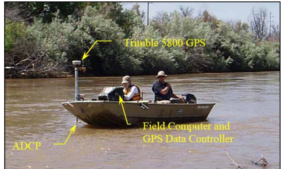
Figure 14: Acoustic Doppler current profiler / GPS setup onboard a boat used in bathymetry surveys in support of Sedimentation and River Channel Studies.
