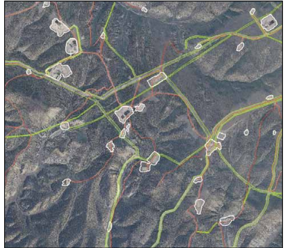
Figure 3: Baseline surface disturbance data for the White River Field Office (WRFO). White polygons represent oil/gas infrastructure; Green represents Right-of-Ways; and Red are Roads and Trails.
