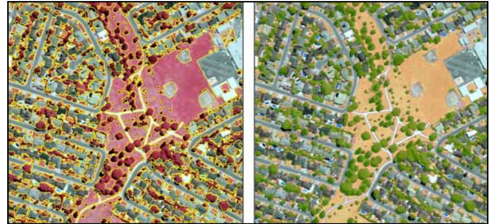
Figure 13: High-resolution imagery utilized in an object-based image processing system allowed maps to be created classifying irrigated turf, irrigated trees/shrubs, and swimming pools supporting consumptive water use studies in the Sacramento/San Joaquin Delta area.
