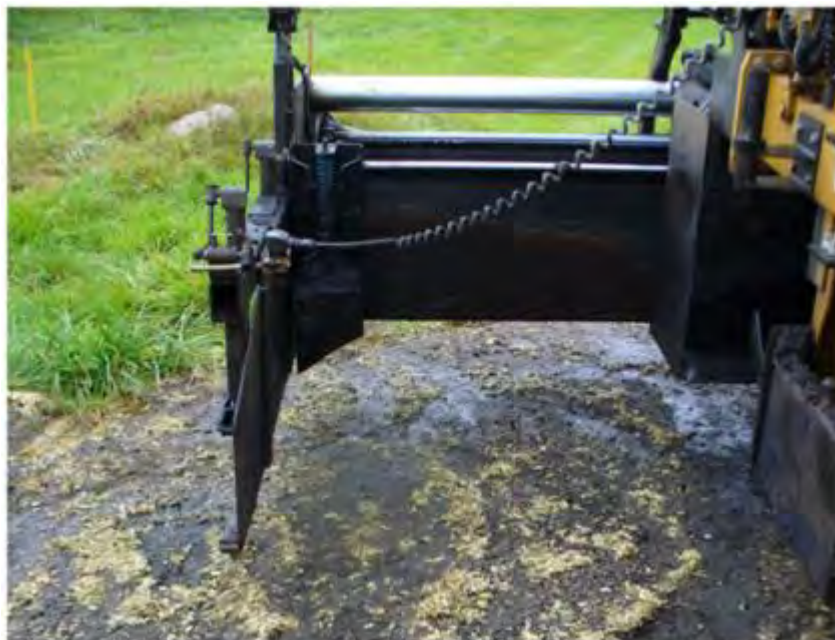
Figure 14. Advant-Edge™ mounted on a paver. Unit is designed to automatically adjust to shoulder elevation changes (driveways and intersections).
