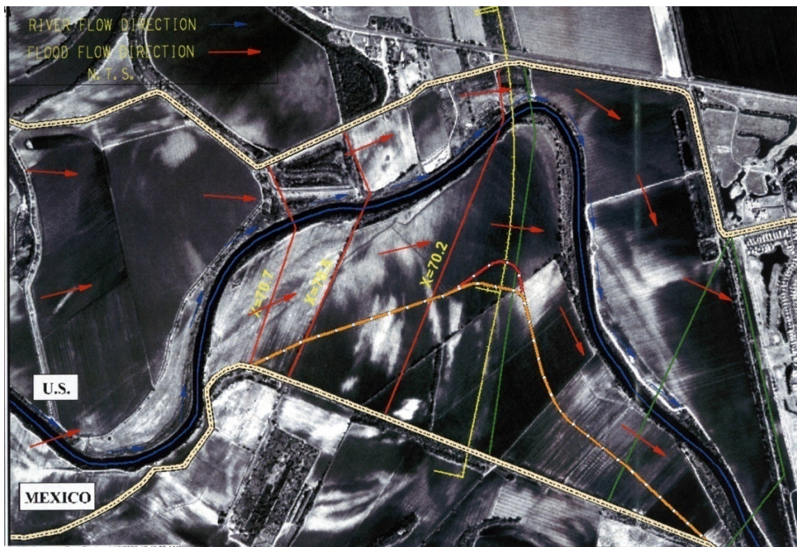
Figure 5.22: River Flow Analysis with current and proposed levees
