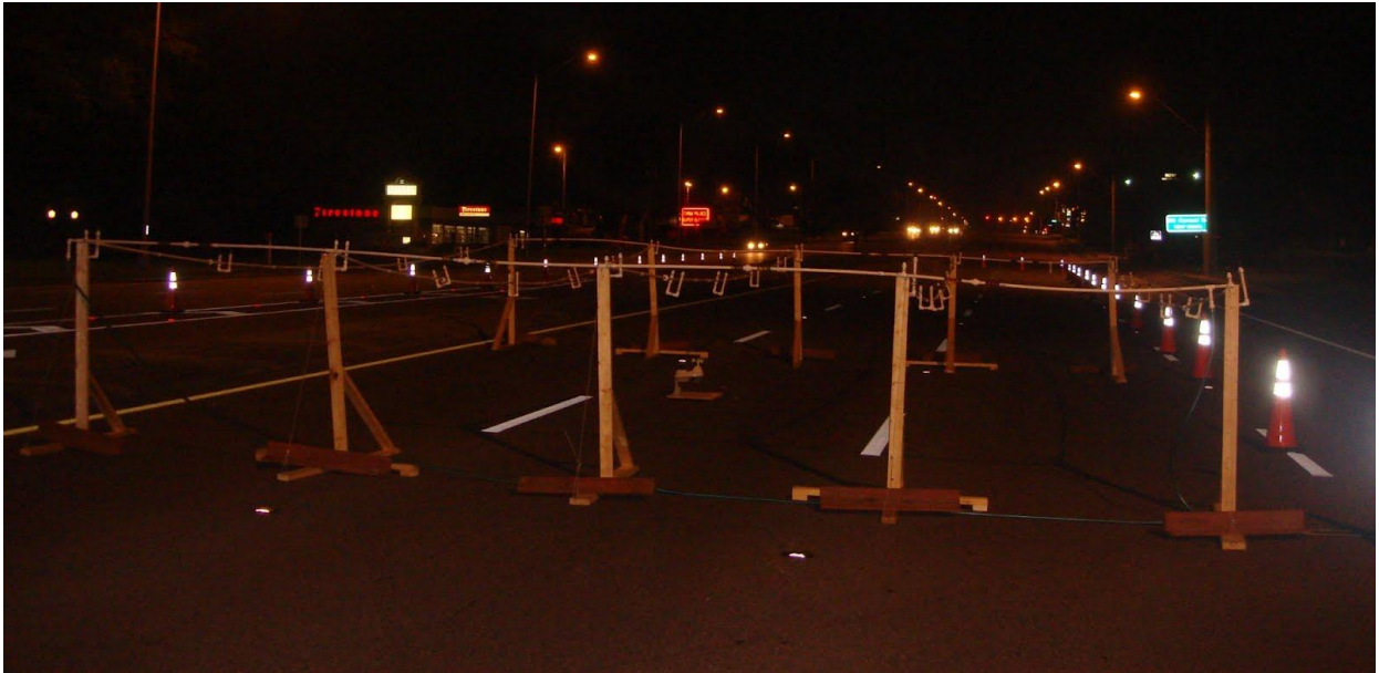
Figure 6.1 Constructed rainfall simulator
