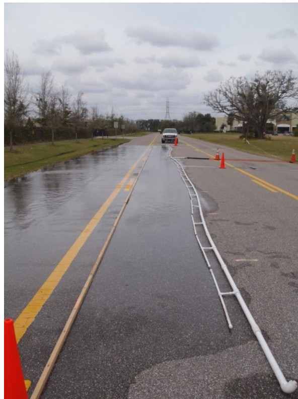
Figure 6.2 Development of water film thickness using water delivery and dam system
