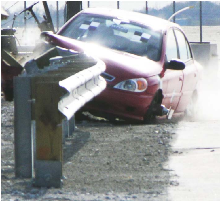
Figure 6. Rail Snag Under Hood of Test No. 2214MG-3
