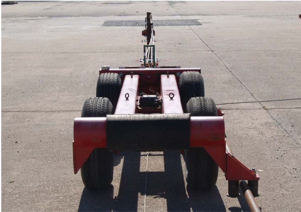
Figure 41. Bogie Test System Setup, Test No. HTCT-1
