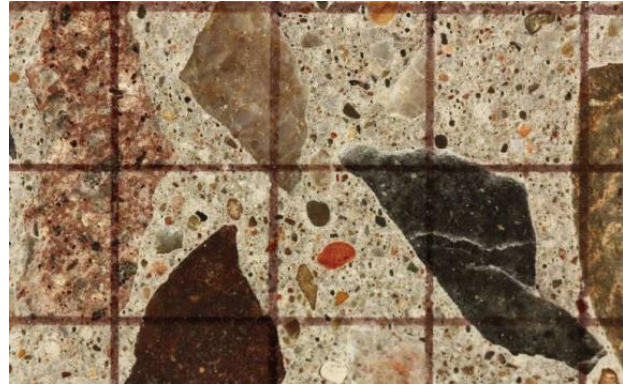
Figure 7.9. Examination of the polished concrete section under the stereomicroscope for the determination of the Damage Rating Index . Petrographic features of deterioration (Table 7.7; Figure 7.4) are counted in a one cm by one cm grid system drawn at the surface of the polished concrete section.
