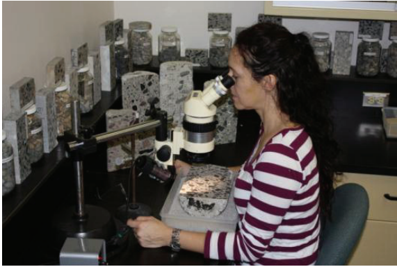
Figure 7.9. Examination of the polished concrete section under the stereomicroscope for the determination of the Damage Rating Index . Petrographic features of deterioration (Table 7.7; Figure 7.4) are counted in a one cm by one cm grid system drawn at the surface of the polished concrete section.
