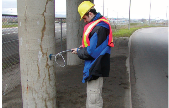
Figure 7.7. In-situ measurements of humidity in concrete. A. Wooden-stick method. B. Vaisala probes.
