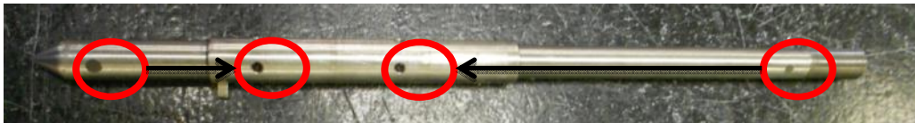
Figure 3-47. First probe modification – repositioned inner rod flow ports
