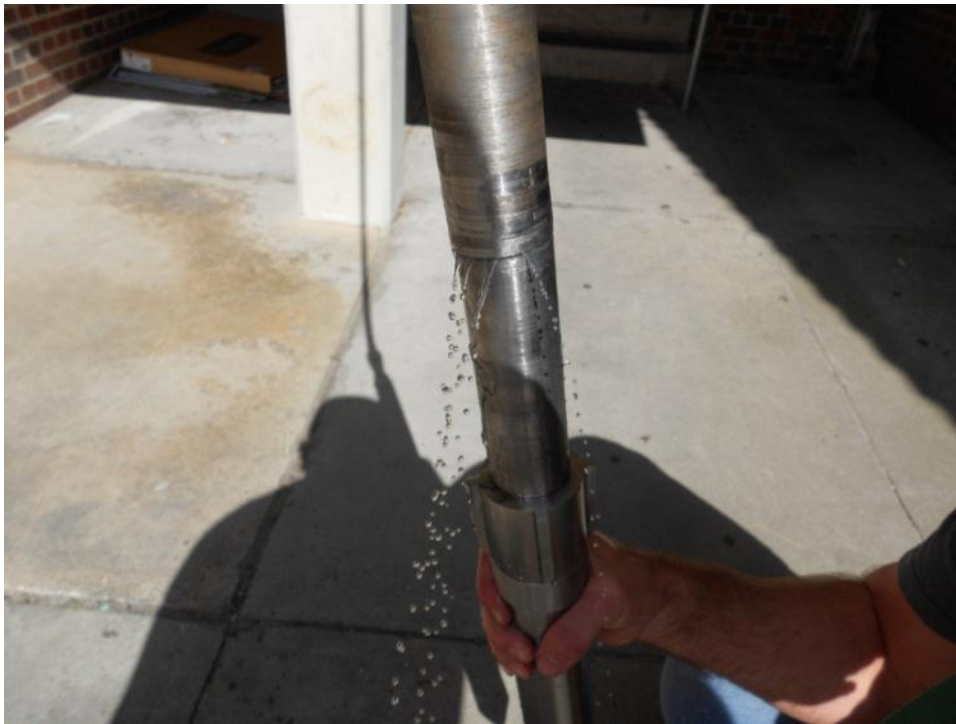
Figure 3-52. AWJ rod connections failing before the probe
