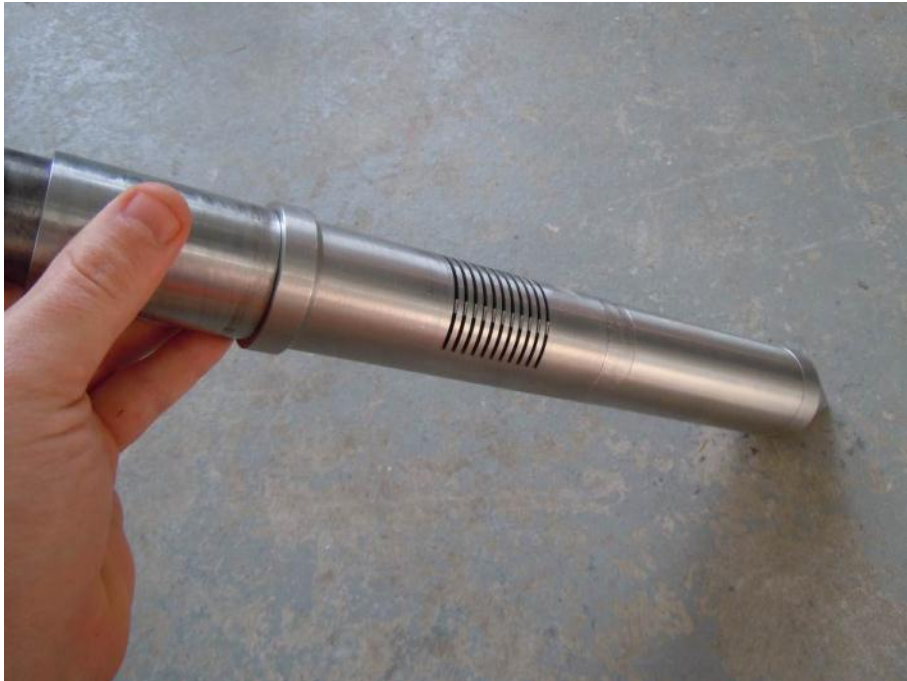
Figure 3-23. Completed smear-resistant VAHIP prototype
