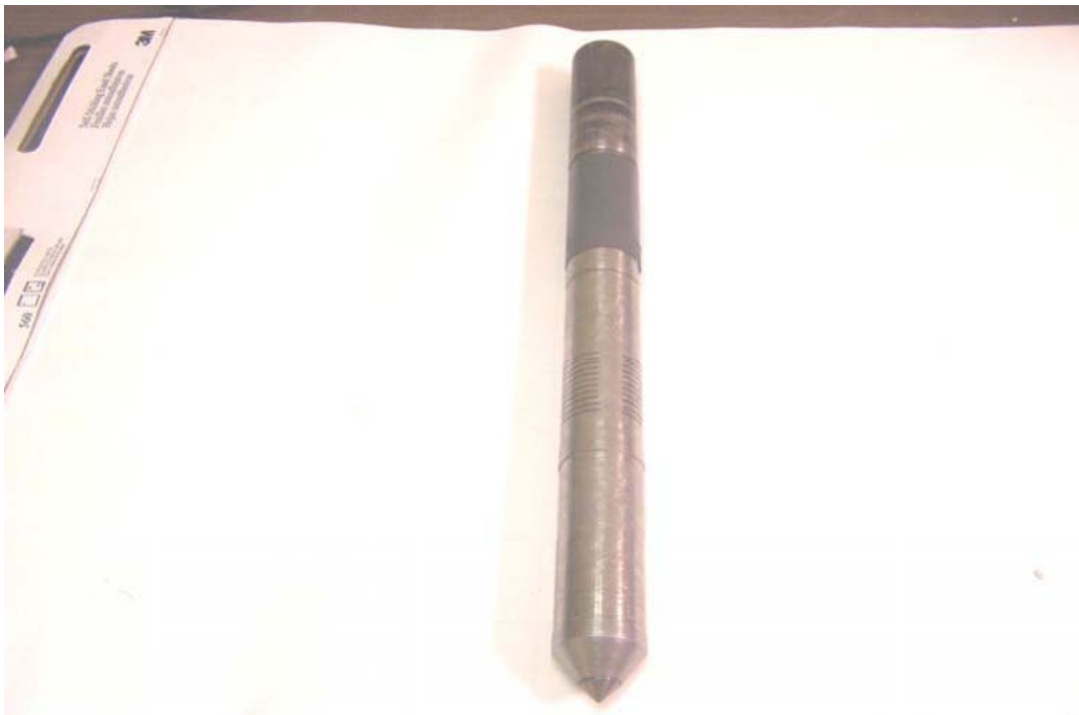
Figure 3-10. Probe tip closed for horizontal flow
