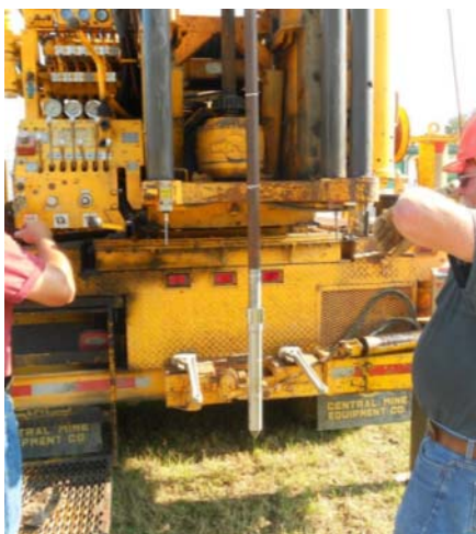
Figure 3-54. Probe attached to the SPT drill rig
