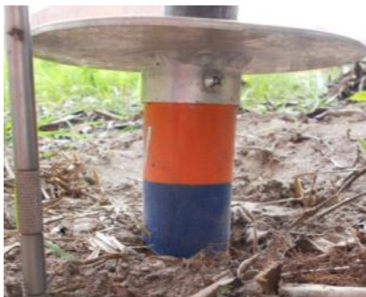
Figure 3-63. Coordinate dial displaying blue section indicating horizontal flow
