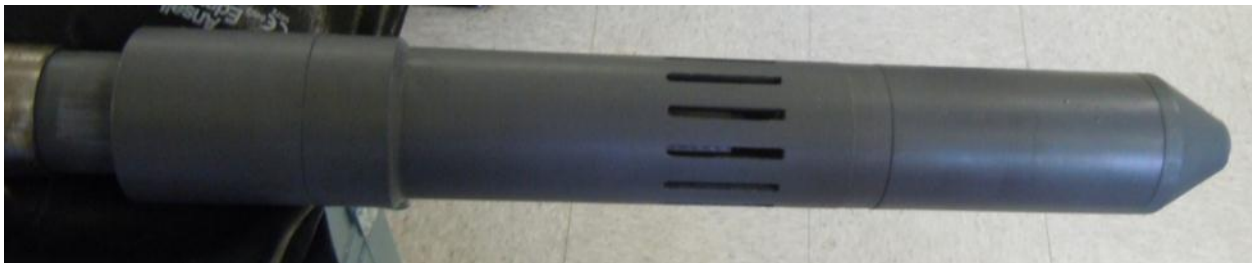
Figure 3-30. First lift stage – horizontal flow
