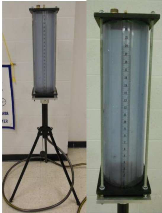
Figure 3-45. New water vessel and support stand
