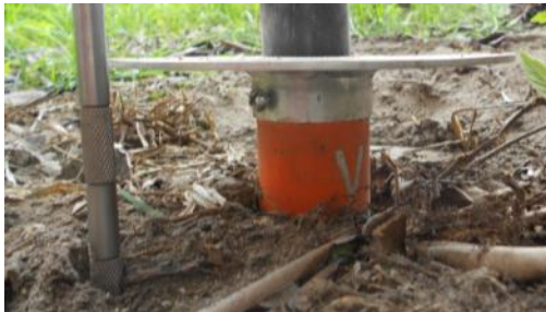
Figure 3-62. Coordinate dial displaying orange section indicating vertical flow
