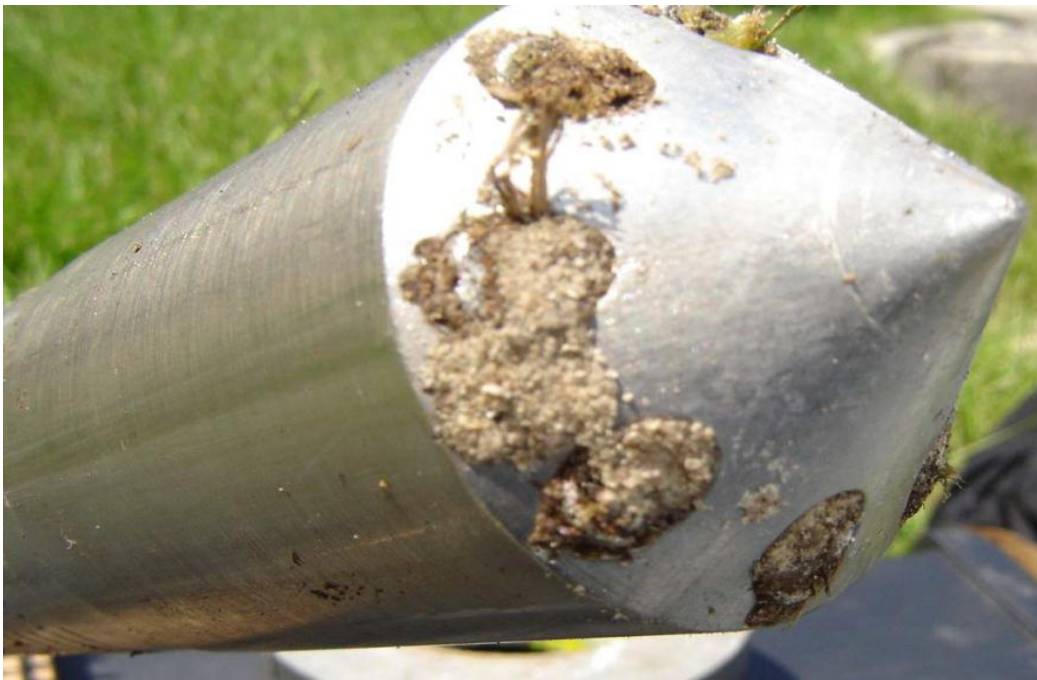
Figure 3-6. Potentially clogged flow ports (2005 probe)
