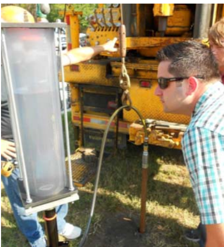
Figure 3-57. Water vessel being monitored for flow
