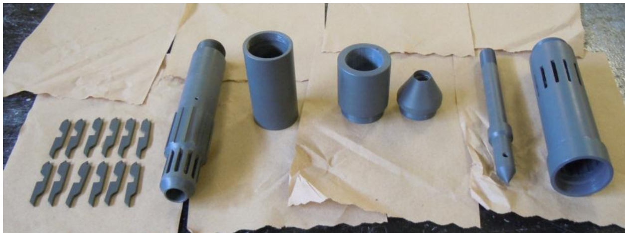
Figure 3-28. Disassembled probe showing individual components
