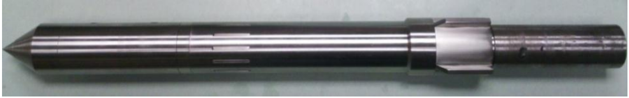
Figure 3-36. New steel probe with AWJ rod attachment
