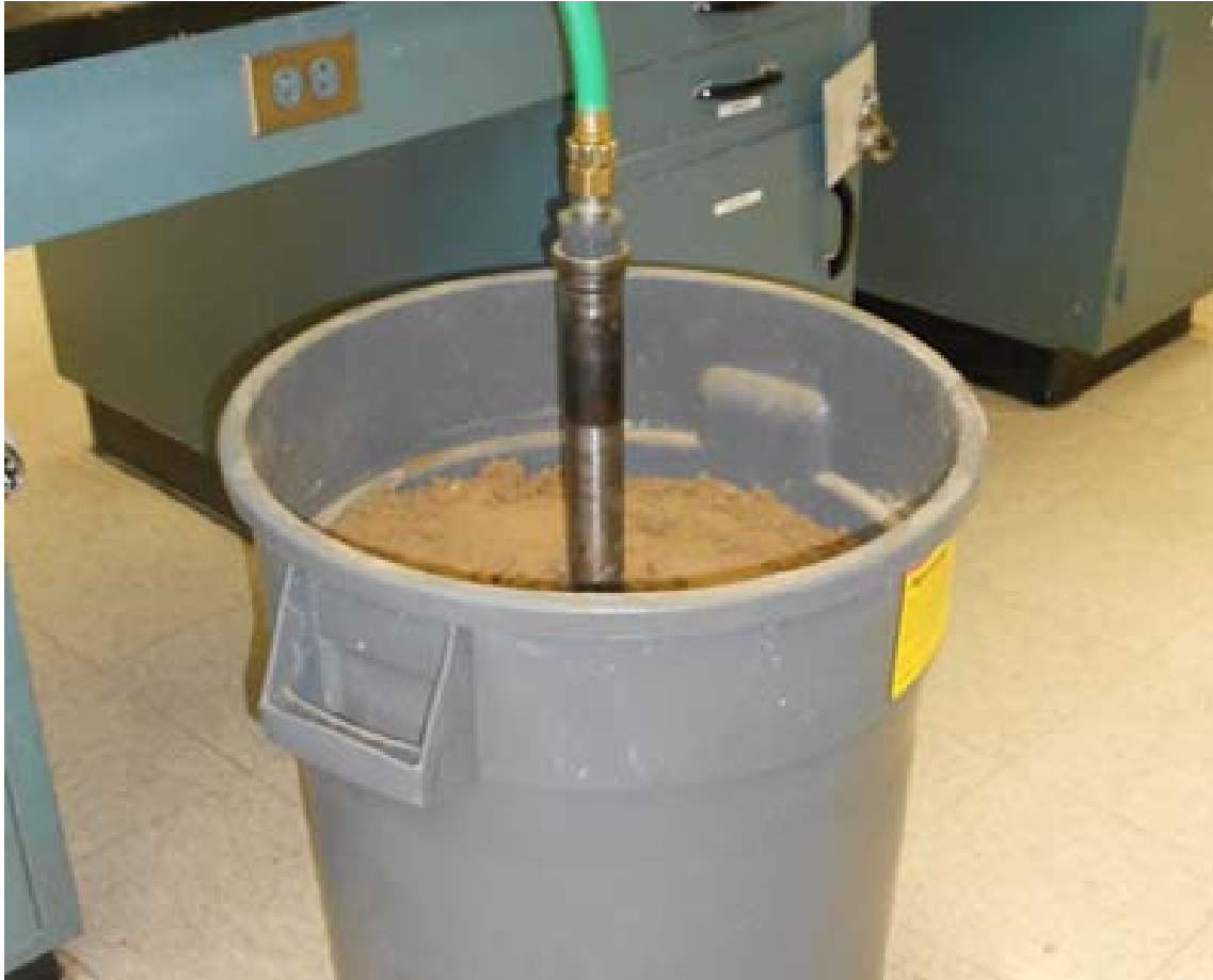
Figure 5-2. Probe embedded in soil
