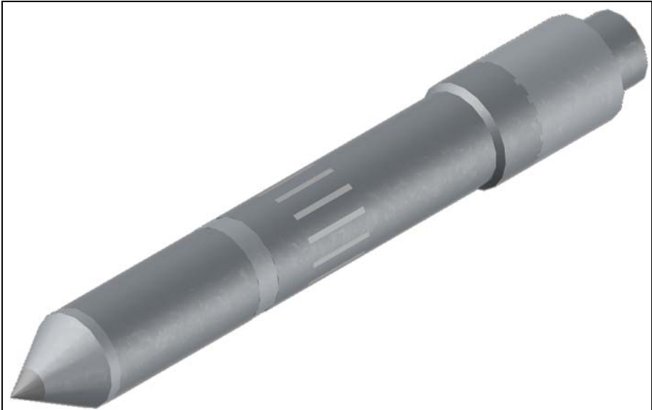
Figure 3-24. Three-dimensional isometric view of new probe design in “closed” position.
