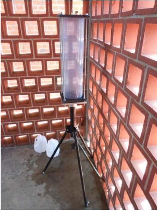
Figure 3-49. Water vessel with 45 foot hose attached on the fourth floor of Weil Hall
