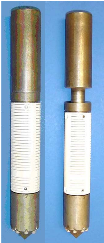
Figure 3-1. VAHIP probe (2004). (A) stage I (vertical permeability); (B) stage II (horizontal permeability)
