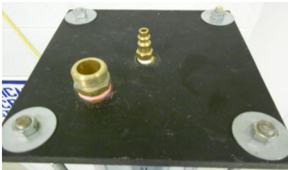
Figure D-4. Top plate of water vessel with removable cap and quick connect
