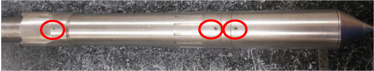
Figure 3-58. Probe with set screws added to prevent unthreading
