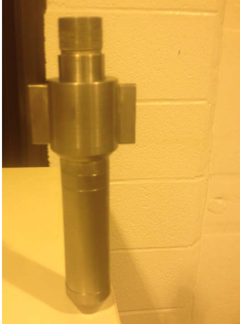
Figure 5-7. Illustration of the VIP's "hanging" outer casing
