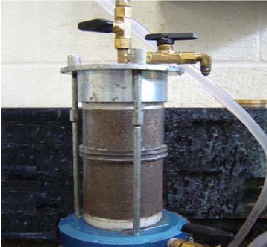
Figure 5-6. Lab permeameter testing permeability
