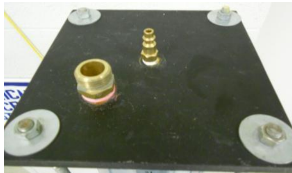
Figure 3-46. Top of new water vessel with standard hose connection and quick connect
