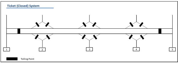
Figure 2-1. An example of a closed system (Dailer and Hevia-Moren 2011a)
