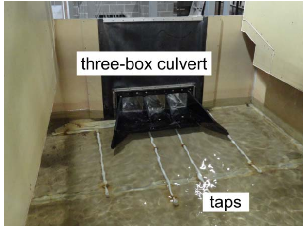
The culvert model without embankment protection
