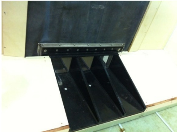
The culvert model with embankment protection
