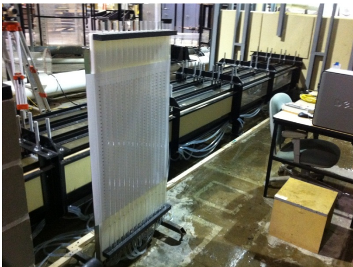
Fig 3-7 Instruments for water surface measurement: a) pressure sensor system, b) in-house developed Labview-based software, and c) manometer
