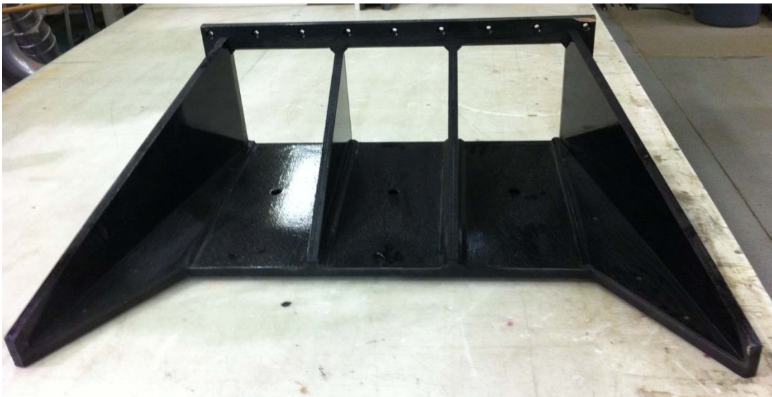
Fig 3-2. The pre-cast culvert model: a) culvert entrance; b) culvert outlet; and c) culvert barrel; d) close view of a detachable culvert inlet
