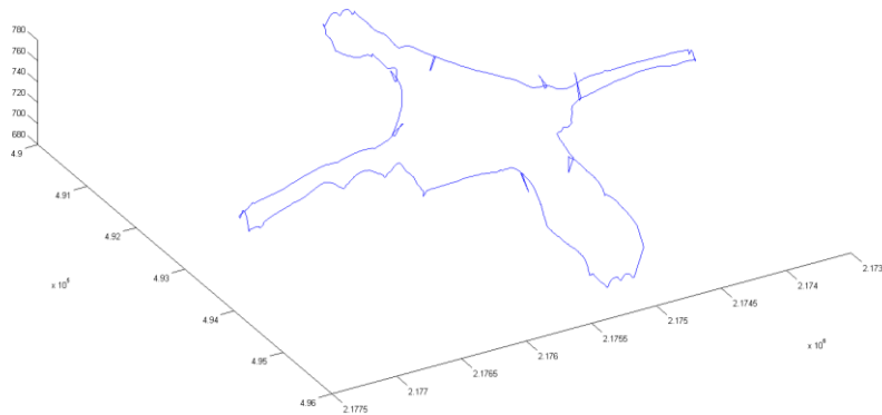
Figure 7. Boundary data “spike” anomalies present in the source data
