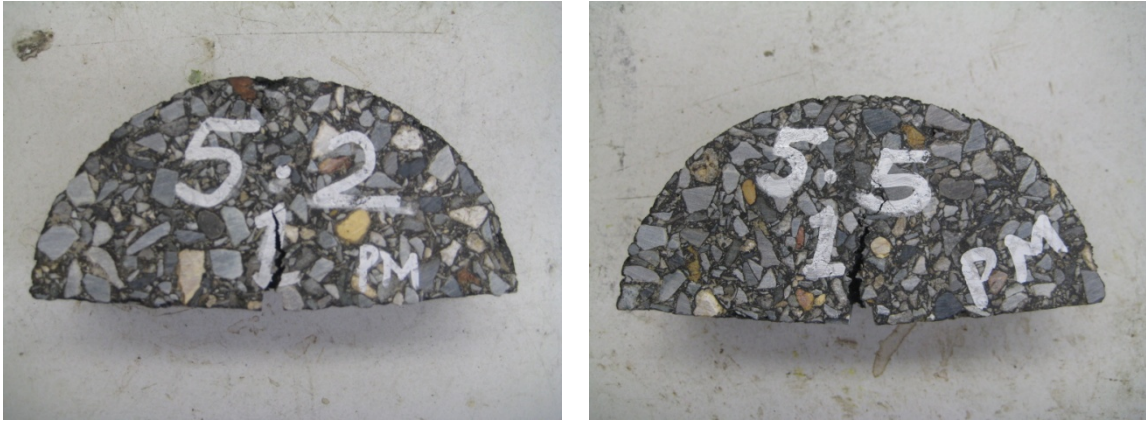
Figure 10. Comparison of 5.2% AC (124 psi) and 5.5% AC (100 psi) SCB Specimens.
