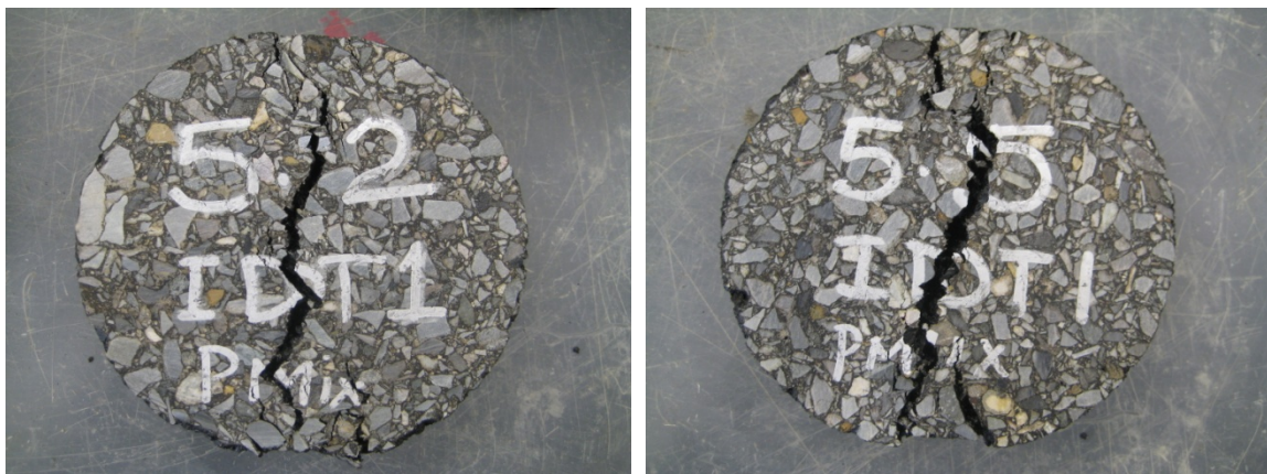
Figure 16. Comparison of 5.2% AC (126 psi) and 5.5% AC (104 psi) IDT Specimens.
