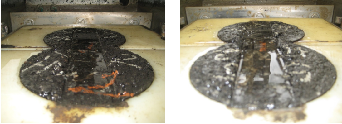
Figure 7. Comparison of 5.2% AC (3.1 mm) and 5.5% AC (4.1 mm) Hamburg Specimens.
