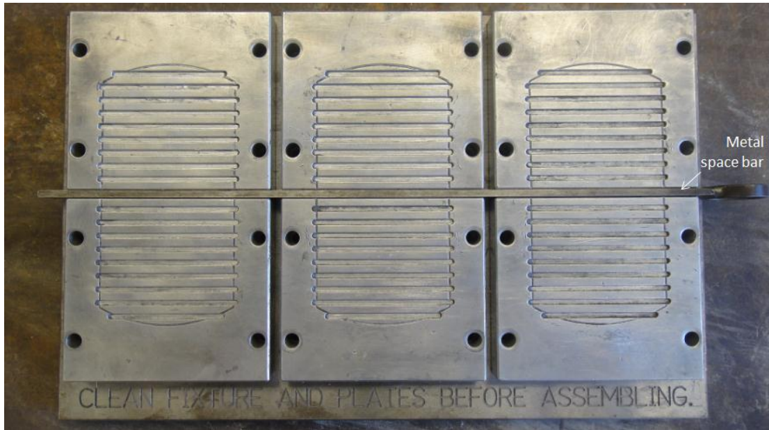
Figure 4. New Mounting Jig and OT Plates with Outer Grooves for Easy Sample Alignment.
