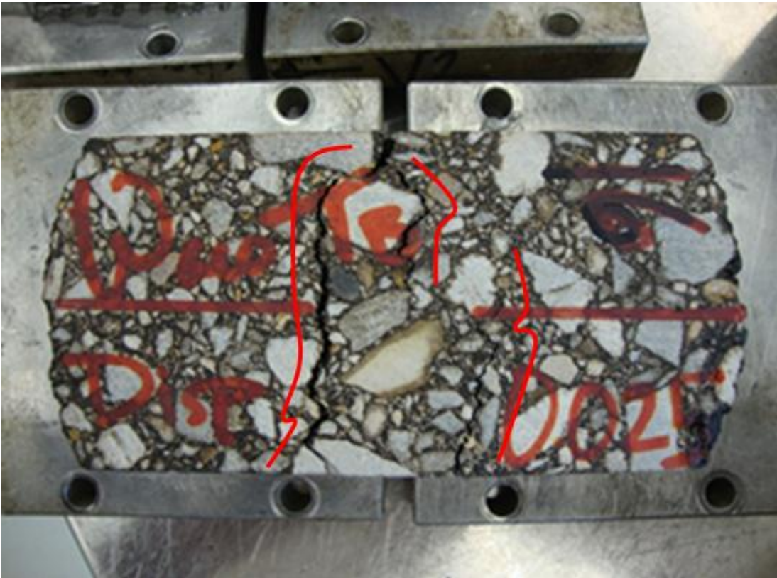
Figure 7b. Example of Double Cracks.
