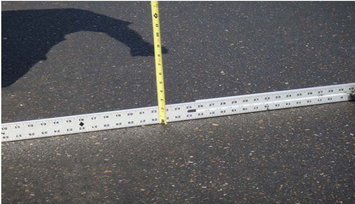
Figure II-1. Surface Rut Measurements with a Straightedge on US 59.
