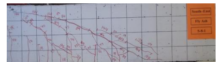
Figure 5.4- Crack pattern of the beams at shear failure (Low cementitious mix)
