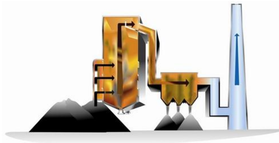
Figure 2.1- Fly Ash Production
