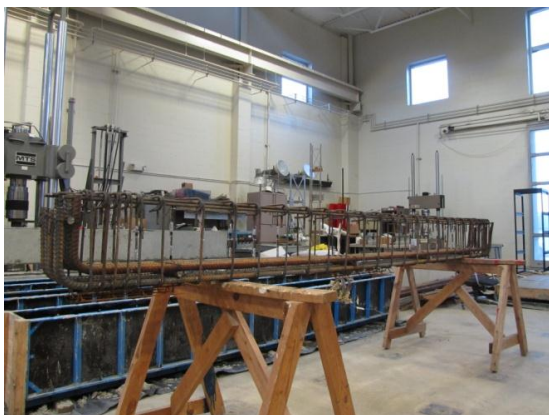
(c) Beams with stirrups in test region
