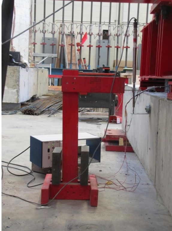
Figure 4.11- Detail of LVDT for Deflection Measurement
